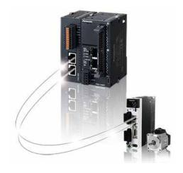
Capable of performing motion control through a high-speed network and supporting an open network with a small PLC
