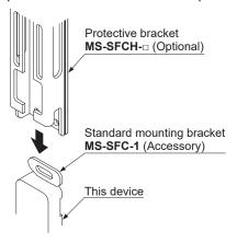
Step 2 Position mounting holes of protective metal Case and standard mounting bracket. And, tighten with two hexagon-socket head bolts [M5 (purchase separately)] on the mounting surface.
