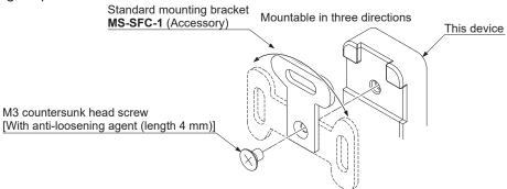
• Install the standard mounting brackets in the mounting surface with two hexagon-socket head bolts [M5 (purchase separately)].
