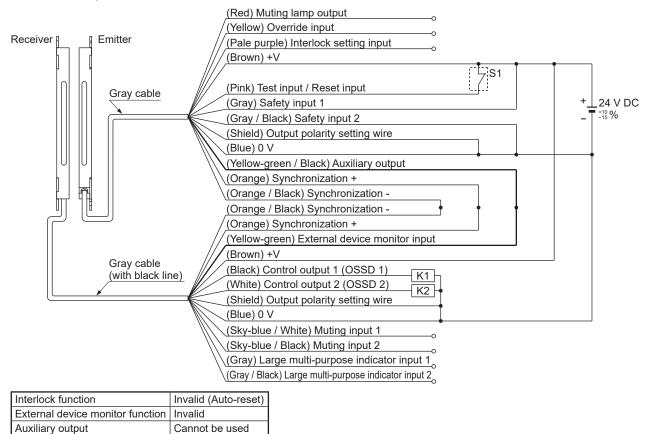
The device output is selected depending on the connecting state of the output polarity setting wire (shield). Incorrect wiring may cause the lockout state.
