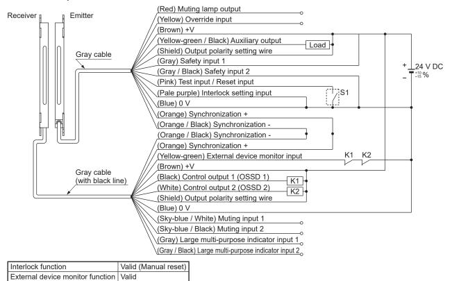
The device output is selected depending on the connecting state of the output polarity setting wire (shield). Incorrect wiring may cause the lockout state.
