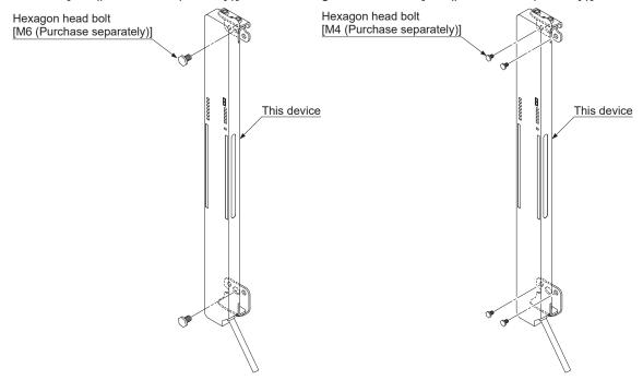
Note: SF4C-H28□ ,SF4C-H32□, SF4C-F55□ and SF4C-F63□ require multifunctional intermediate supporting bracket MS-SFC-4 (optional).
