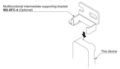
Step 2 Set the multifunctional intermediate supporting bracket on the mounting surface using a hexagon head bolt [M6 (purchase separately)] or a hexagon-socket head bolt [M6 (purchase separately)].
