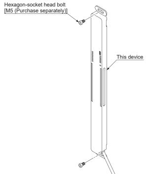
Note: The case of the product is made of resin so the longitudinal dimension is subject to expansion and contraction. When drilling mounting holes, check the drilling locations by positioning the actual product at the installation location.
