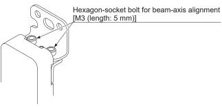
Step 4 Change direction of the part A of multifunctional mounting bracket. And tighten the two of hexagon-socket head bolts for beam-axis alignment M3 (length 5 mm)]. The tightening torque should be 2 N·m.
