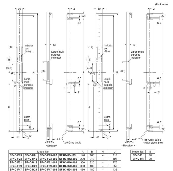
Notes: 1) Measurement of drawing above is indicator part of SF4C-H□ SF4C-H8□ and SF4C-F15□ are not provided with digital error indicator (red).
