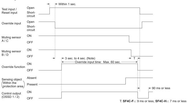
Note: This is when the muting lamp diagnosis function is valid. If the muting lamp does not light up even if 1 sec. or more is passed, the override function becomes invalid. When the muting lamp diagnosis function is invalid, the override function becomes valid 3 sec. after the input conditions of the muting sensor A (C) and B (D) were satisfied.
