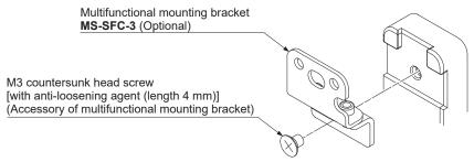
Step 3 Set the multifunctional mounting bracket on the mounting surface using either two hexagon-socket head bolts [M6 (purchase separately)] or four hexagon-socket head bolts [M4 (purchase separately)].
