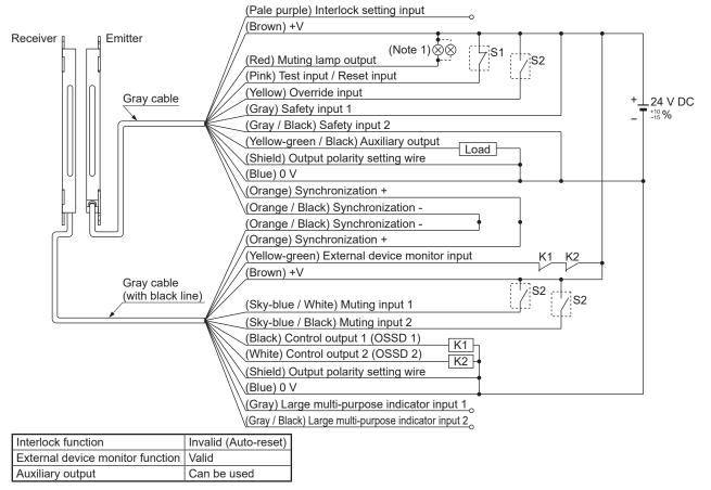
The device output is selected depending on the connecting state of the output polarity setting wire (shield). Incorrect wiring may cause the lockout state.
