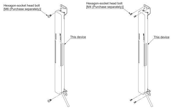
Note: SF4C-H28□ ,SF4C-H32□, SF4C-F55□ and SF4C-F63□ require multifunctional intermediate supporting bracket MS-SFC-4 (optional).
