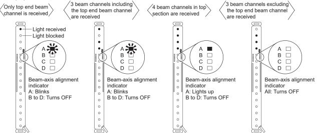
When all the 4 beam channels divided into each section are received, the beam-axis alignment indicator lights up in red. The indicators corresponding to the different sections light up in red, one by one, when the beam channels of the respective sections are received. When all the beam channels are received and the control output (OSSD 1 / 2) turns ON, all the four indicators of the beam-axis alignment indicator turn into green.
