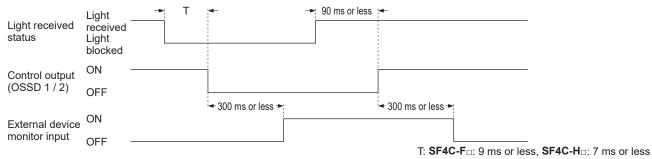
The setting time of the device monitor is 300 ms or less (Note). Exceeding 300 ms turns the device into lock-out status.
